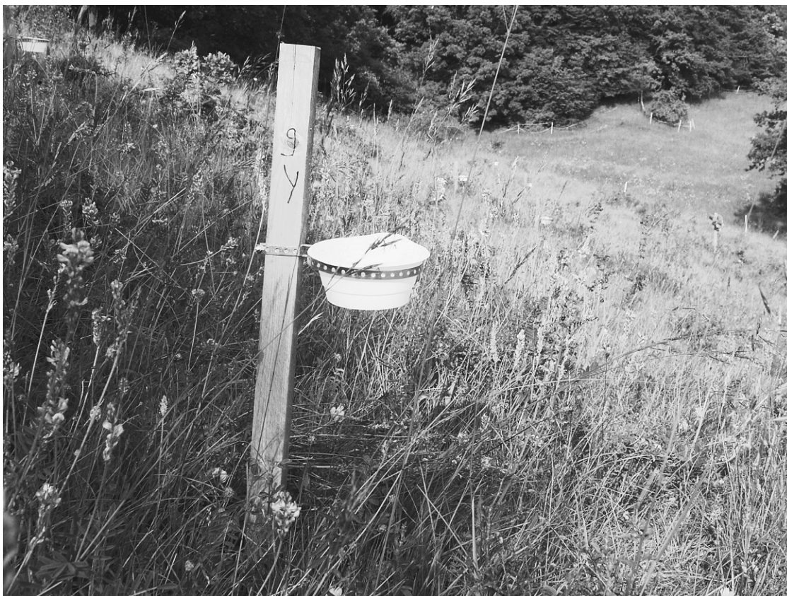
PLATE 1. Experimental setup on a calcareous grassland in Germany (Huhnsberg, Scheden). The UV-bright pan traps (shown in the foreground) represented the most effective method in detecting bee species richness and thus can be recommended for pollinator monitoring schemes. Trap nests (shown in the background) can be used as a complementary method to detect additional cavity-nesting bee species. Photo credit: C. Westphal.
